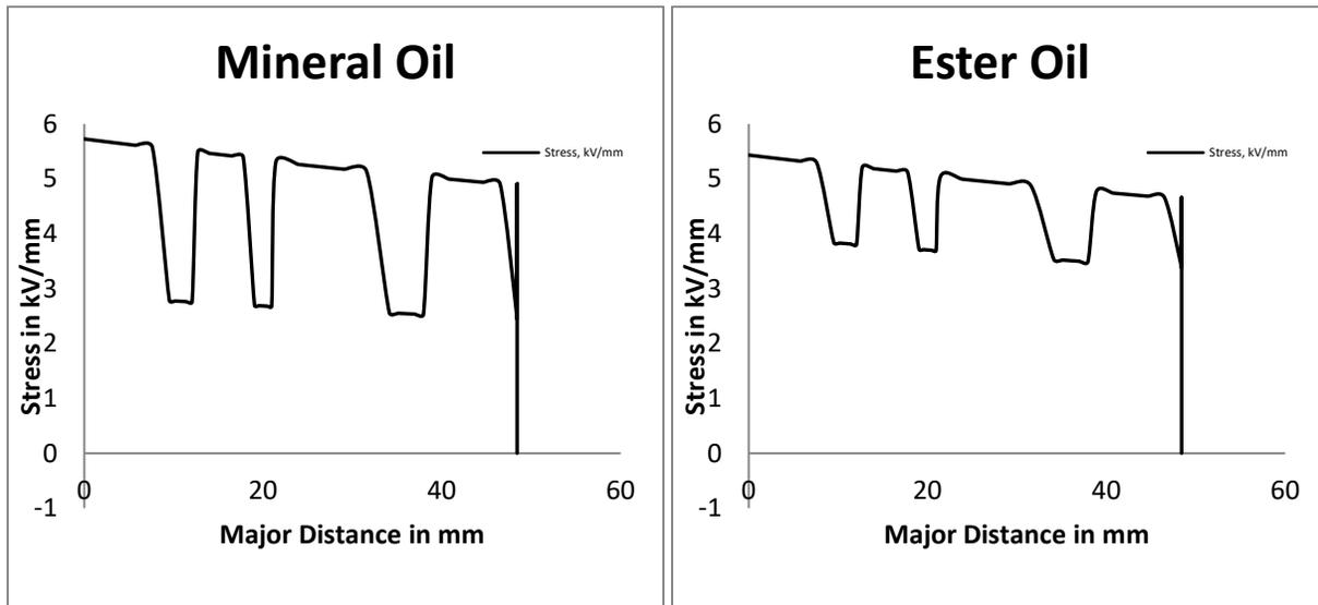
Due to stress shift from the liquid to solid insulation, stress in high voltage leads can be challenging for the stress control. Radial insulation on the lead shall be evaluated by the trade-off between electrical and thermal requirement. Comparison of lead stress between mineral oil and FR3 fluid tabulated below.
