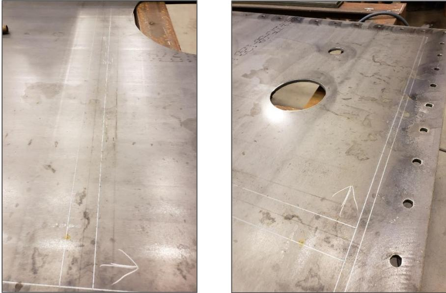
The location of parts used to be layed out by using tape and later laser measurements. This was time consuming and prone to errors. The location of the part is 'etched' on the steel plate with a tungsten carbide mounted to the X Y traveling arm. The arm is driven by a the DXF file from the 3D CAD design. The example shows Etched top cover for bracing location marked. The lines are produced by the scribing on the plate.
