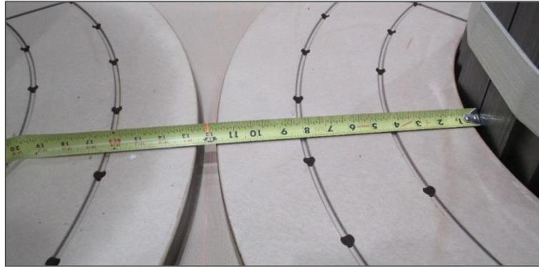
Using the Measuring tape, take measurements at the bottom and the top of the core leg in the core window. These methods are employed to check manufacturing tolerances; if these tolerances are not met, then engineering and Quality is to be consulted before proceeding.
