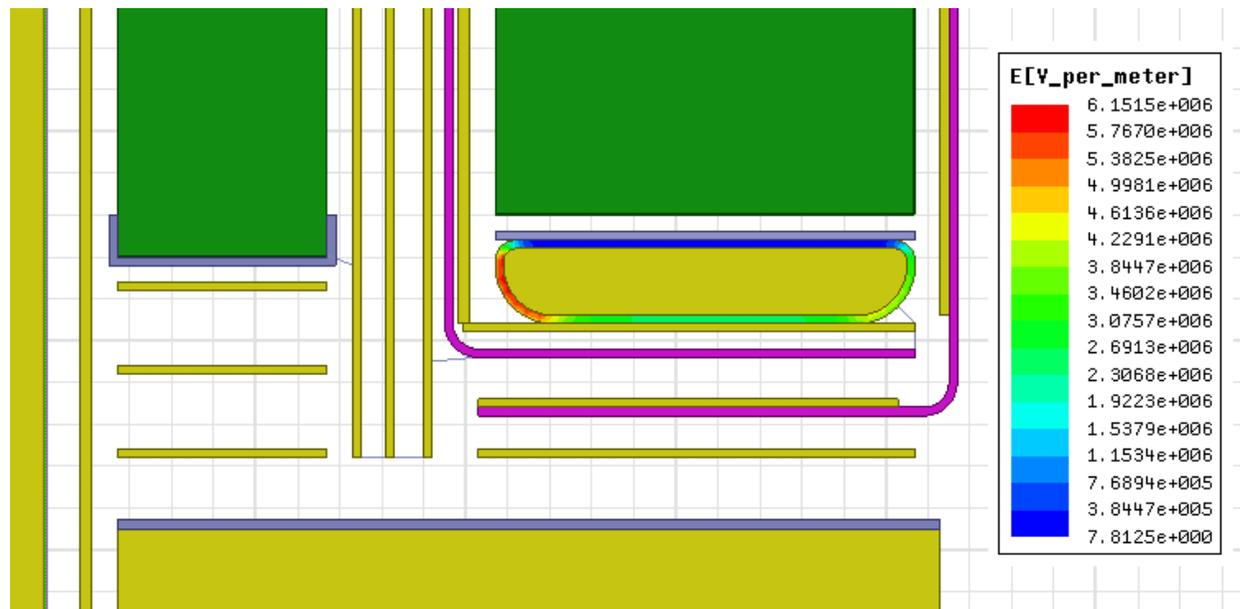
**Fig. 1 Electric Field Plot of Insulation Structure of a High Voltage Transformer.**
