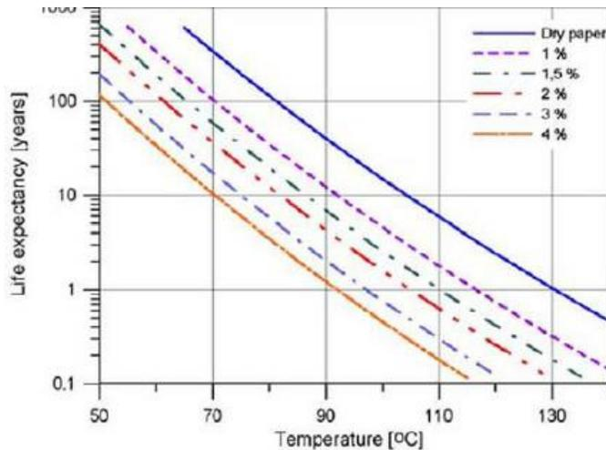
**Fig 2. Moisture directly Affects Life of the Insulation**
