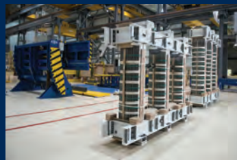
Core stacking area
