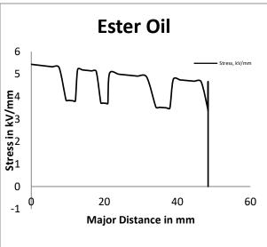
Due to stress shift from the liquid to solid insulation, stress in high voltage leads can be challenging for the stress control. Radial insulation on the lead shall be evaluated by the trade-off between electrical and thermal requirement. Comparison of lead stress between mineral oil and FR3 fluid tabulated below.
