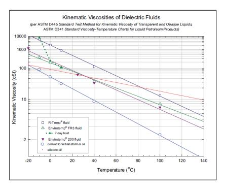
Figure 1. Viscosity of different fluids
