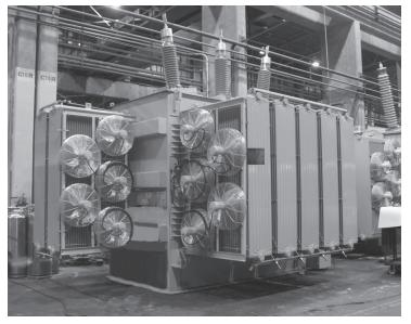
One of two 120 kV/ 25 MVA transformers built for NASA Ames Supercomputing facility
